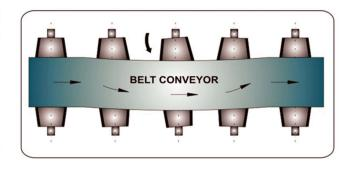
The degree of pivot of the Tracker Roller depends on how far the belt deviates from the center. As the Tracker Roller is no longer perpendicular to the return belt's direction, this skewed roller automatically guides the belt back to its central position.
